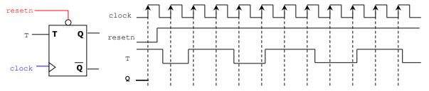
b) Complete the timing diagram of the circuit whose VHDL description is shown below: (5 pts)
